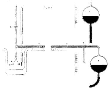
A flat membrane of the material to be studied closes the 15.0 mm. in diameter opening of the brass holder A and is held in place by the stout ring B, which is drawn up tightly by three screws<sup>3</sup>. The metal bearing on
